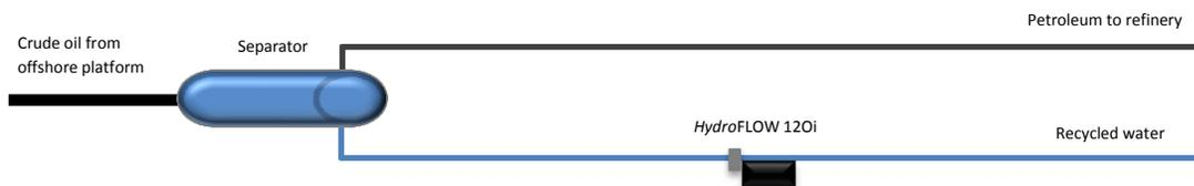
**Goal of product evaluation:** Reduce scale accumulation inside the pipe and possibly soften existing scale deposits. The scale is predominantly made up of iron. In addition, lab analysis of the scale detected small quantities of magnesium, calcium carbonate and silicon.
